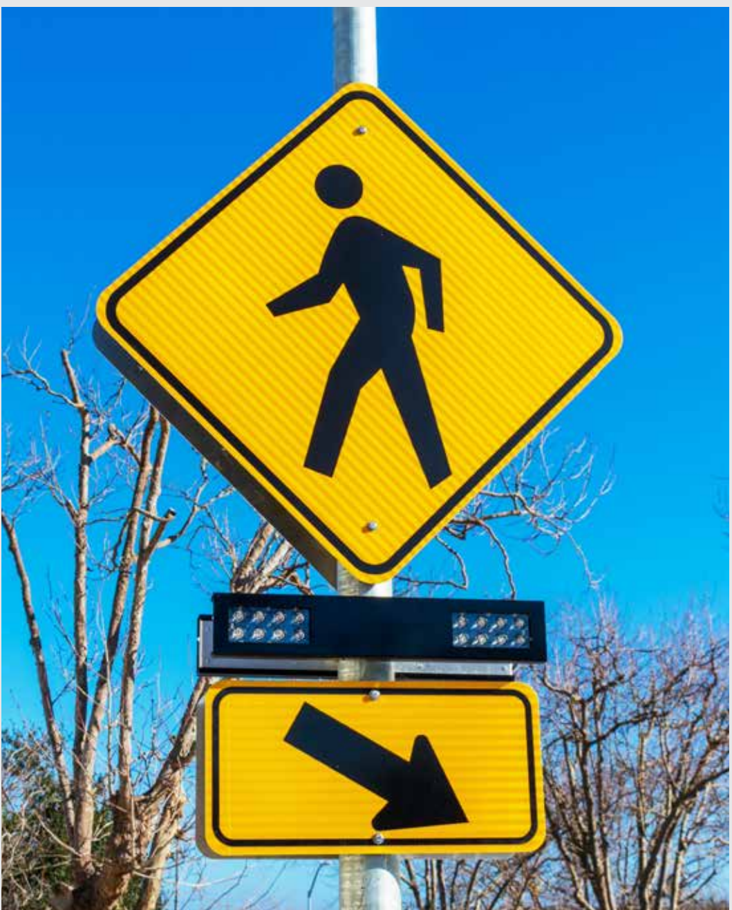
Rectangular Rapid Flashing Beacon (RRFB)
