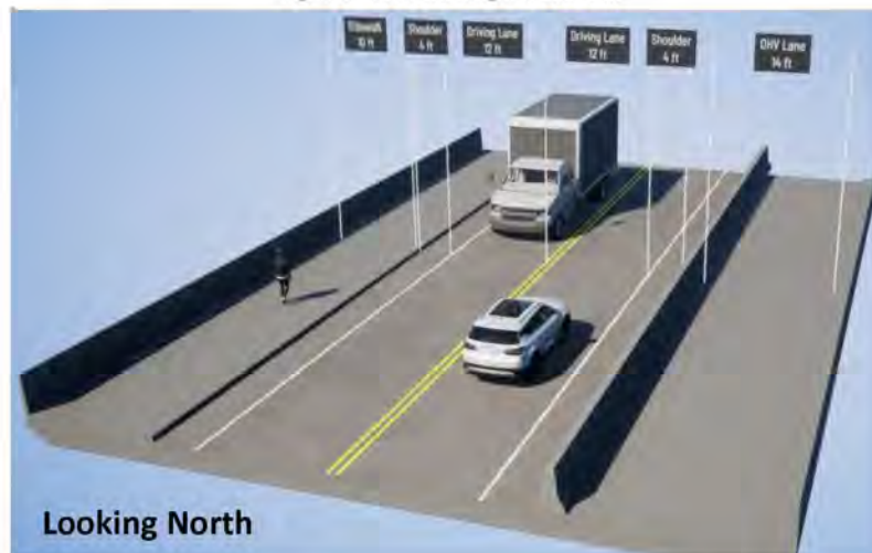
Figure 3 – CSAH 100 Bridge Cross Section
