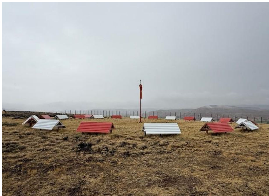
Figure 2-1– DUB Windcone and Segmented Circle
